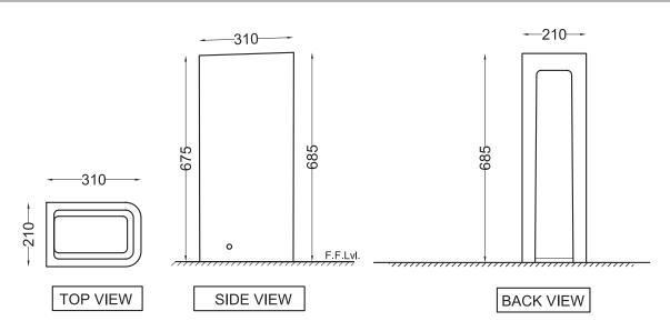
ALL DIMENSIONS ARE IN MM. (TOLERANCE ± 5 MM)
